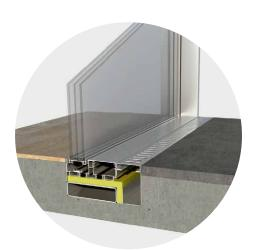
Thanks to the thin profiles and concealed threshold, a continuous line can be maintained between the indoor and outdoor floors.
